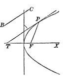
of PFX: therefore, the triangle PTF is isosceles, and consequently PT is tangent to the curve at P.
